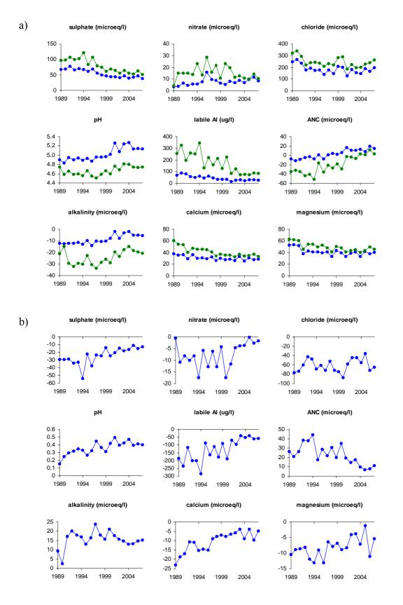
Figure 3.24 a) Comparison of mean annual chemistry time-series for a range of key determinands at the moorland site Round Loch of Glenhead (blue) and the neighbouring afforested site Loch Grannoch (green) in Galloway, southwest Scotland; b) time-series of the difference between annual mean levels for Round Loch of Glenhead and Loch Grannoch
