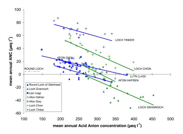
Figure 3.27. Comparison of relationships between annual mean ANC and the sum of annual mean acid anion concentration (i.e.  $[SO_4^{2-}] + [NO_3^{-}] + [C\Gamma]$  for the afforested and non-afforested pairs. Llyn Cwm Mynach is excluded from the plot due to uncertainties associated with ANC estimates for the site. Lines fitted by linear regression.
