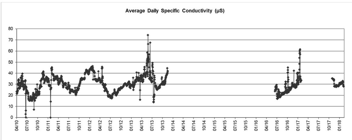
Probe removed Feb 2017 and replaced Nov 2017. Conductivity data gap due to probe malfunction
