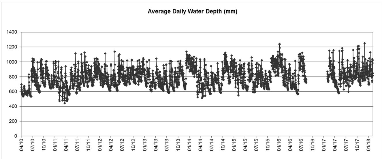
Data gap due to probe malfunction
