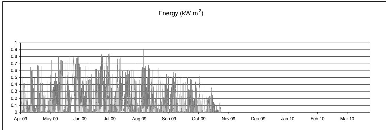
Data gap due to station malfunction.
